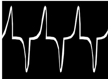
**Figure 5** Synthesized Non-Linear current waveform. Crest Factor ~ 2.4
