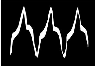
**Figure 4** Actual computer load current waveform. Crest Factor ~ 1.9
