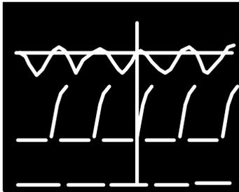
TOP TRACE: Full Wave Rectified Input Waveform
